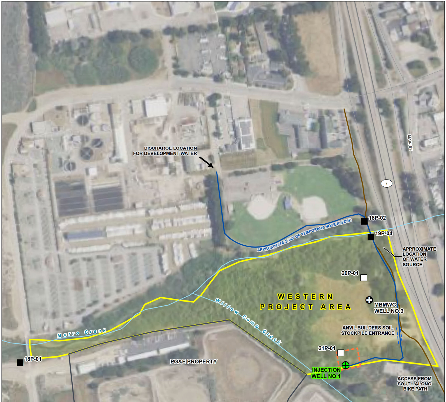
FIGURE 1 Proposed Initial Injection Well Location Map Morro Bay Indirect Potable Reuse Program Injection Testing
