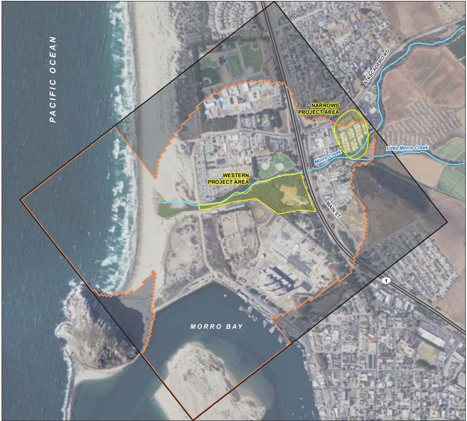
FIGURE 4 Numerical Model Domain Characterization and Selection of Project Areas for Injection Testing
