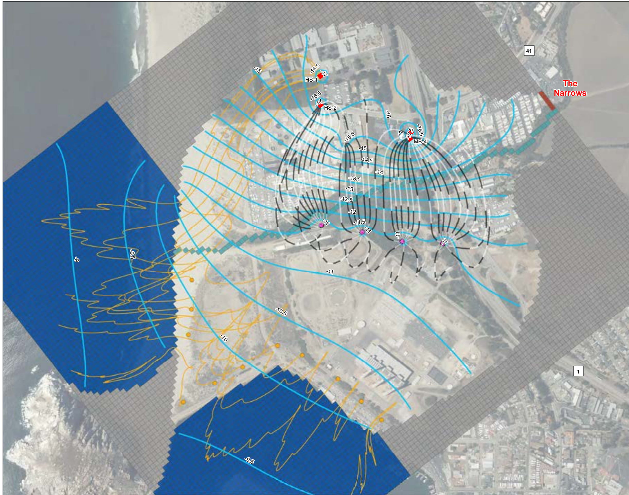
FIGURE 13 Recycled Water Response Retention Time Scenario 2B During Dry Periods Morro Bay, California
