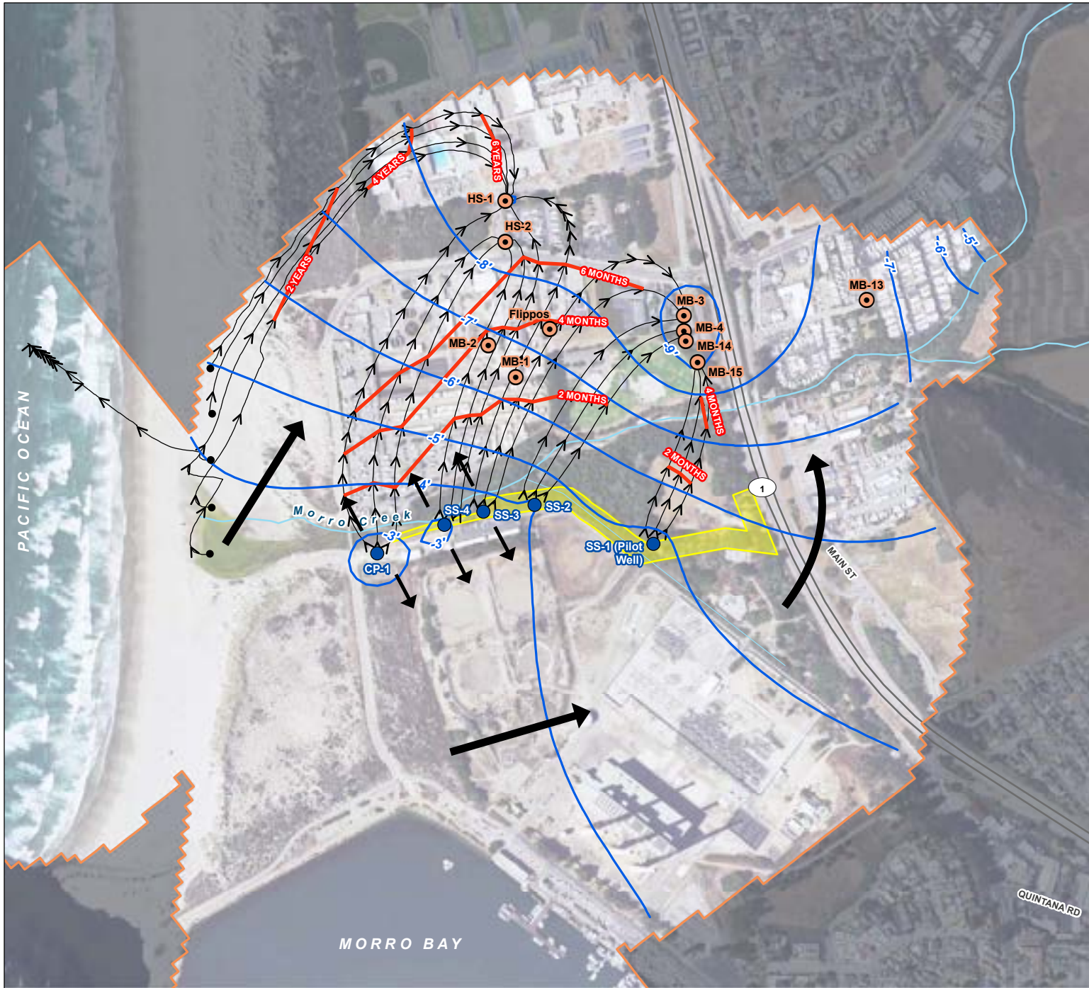
FIGURE 3 Scenario 1 Model Results – Dry Period Morro Bay IPR Project Groundwater Modeling Scenarios 1-4
