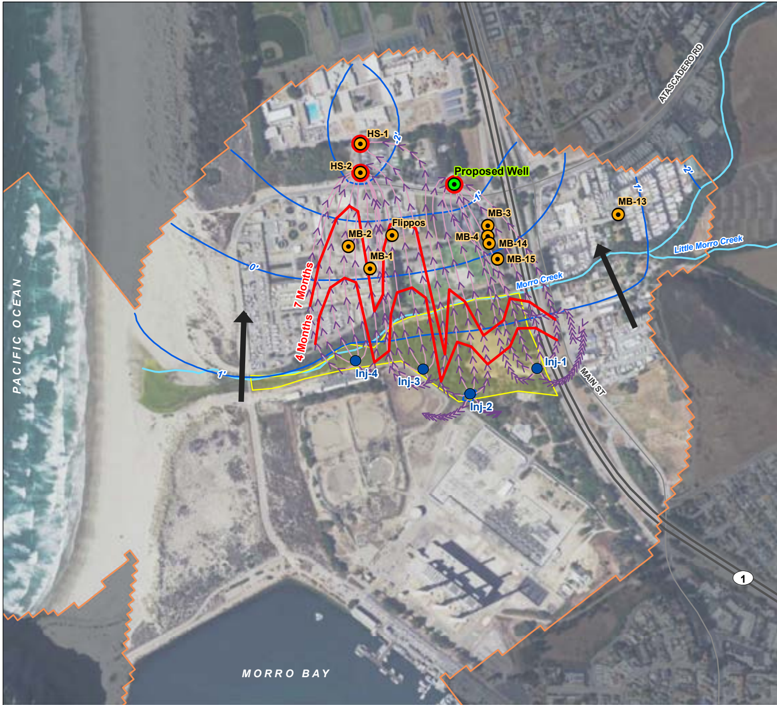
FIGURE 8 Scenario 1C: Groundwater Elevations and Retention Time, Dry Conditions Western Project Area Phased Implementation Scenarios
