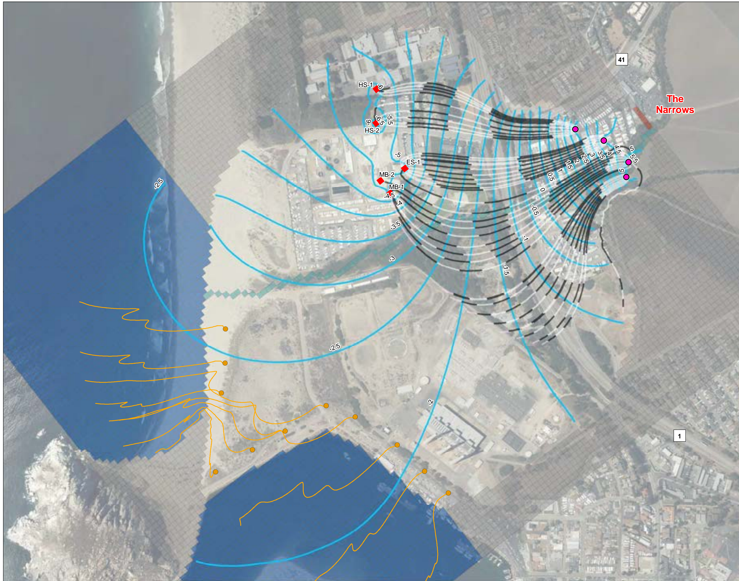
FIGURE 7 Recycled Water Response Retention Time Scenario 1A During Dry Periods Morro Bay, California
